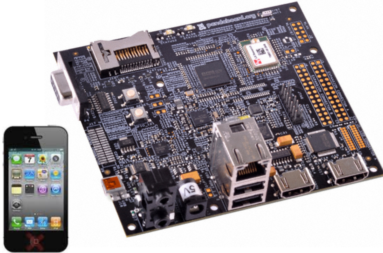
PandaBoard – TI OMAP4, dual core ARM, PowerVR GPU
