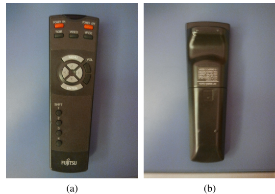
Fig. 5: The top and bottom of the television remote. The support distribution of the remote is much more complex than a simple polygon. Additionally the narrow end is significantly more massive than the wider end owing to the batteries inside.
