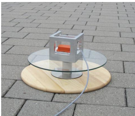
Fig. 3: A high precision aluminum cube on a turntable made of glass and aluminum with a flat wooden plate as a leveled base served as test setup for performing known motions. Here, the Xsens MTi is mounted inside the cube.
