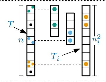
**Step 1:** Insert everything into a hash table, *T*, of size *n* using a weakly universal (w.u.) hash function, *h*  **Step 2:** The  $n_i$  items in T[i] are inserted into another hash table  $T_i$  of size  $n_i^2$  using w.u hash function  $h_i$  **(Step 3)** *Immediately repeat if either* a) *T* has more than *n* collisions
