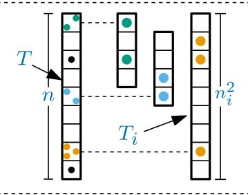
**Step 1:** Insert everything into a hash table, *T*, of size *n* using a weakly universal (w.u.) hash function, *h*  **Step 2:** The  $n_i$  items in T[i] are inserted into another hash table  $T_i$  of size  $n_i^2$  using w.u hash function  $h_i$ (**Step 3**) *Immediately repeat if either* a) *T* has more than *n* collisions b) some  $T_i$  has a collision
